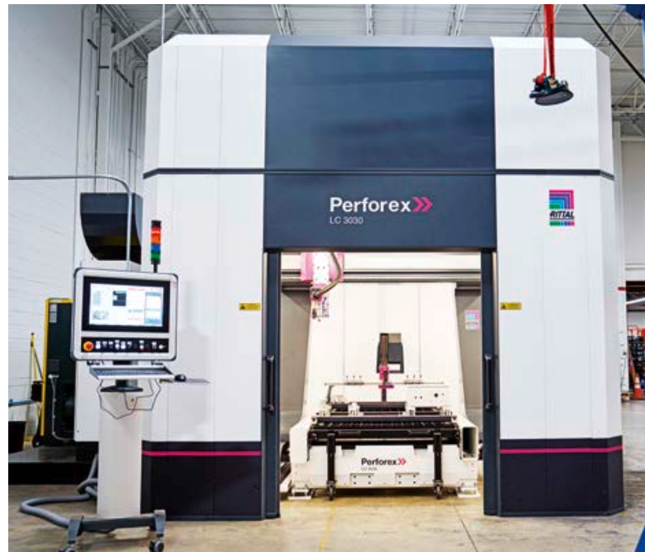
The Rittal Perforex laser centre LC – ideal for the automated mechanical modification of standard enclosures made of stainless steel, sheet steel and powder-coated metals.
