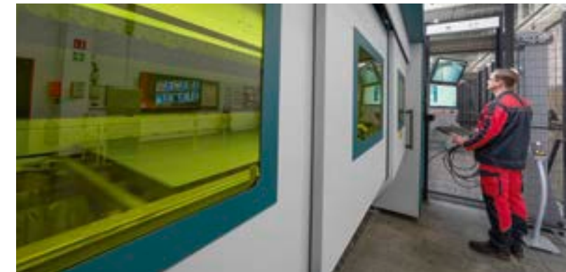
The new laser cutting unit cuts any required shape from sheet metal, in any batch size.
