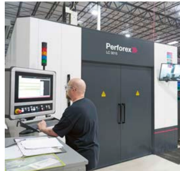
The Perforex LC laser centre is ideal for the automated mechanical modification of stainless steel and sheet steel enclosures.
