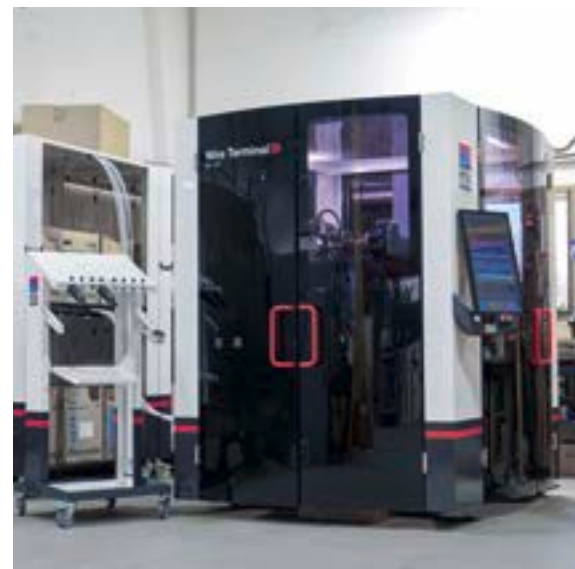
Usemco uses the Rittal Wire Terminal WT C for fully automated wire processing.
