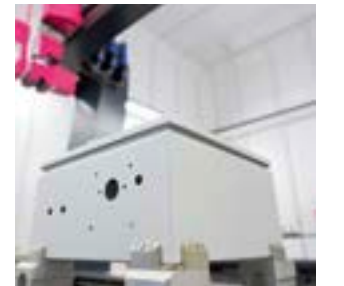
Below: Enclosures are modified with speed and precision thanks to laser technology.
