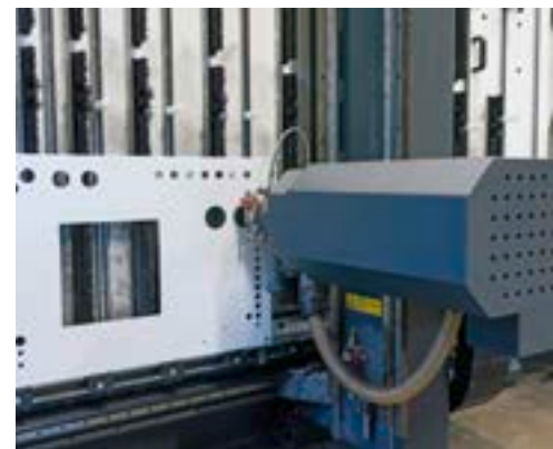
A Perforex BC from Rittal is used to machine enclosures and busbars on the basis of Eplan data.
