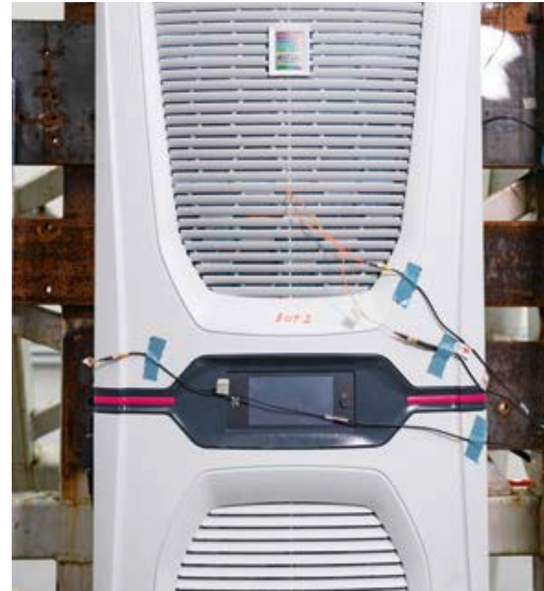
Put through its paces: Vibrations that are produced on a ship by the diesel engine are recreated under laboratory conditions, and their impact on the cooling units is measured.
