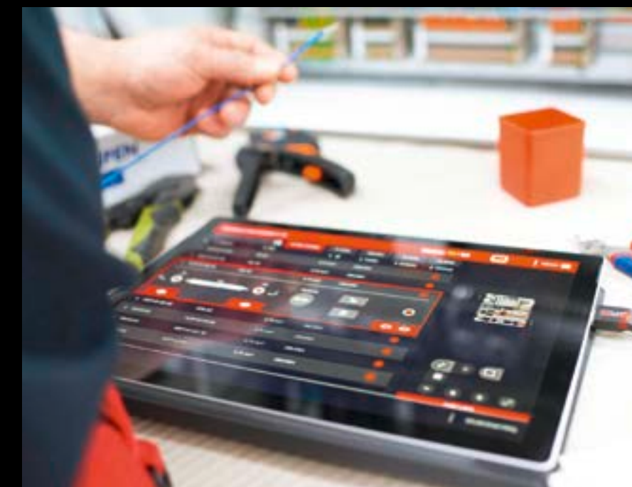
Eplan Smart Wiring: This software is a virtual assistant for manual wiring in enclosure assembly. From the connection point through to the exact routing, the software provides all the wiring information you need – in digital form and also in 3D, if required.
