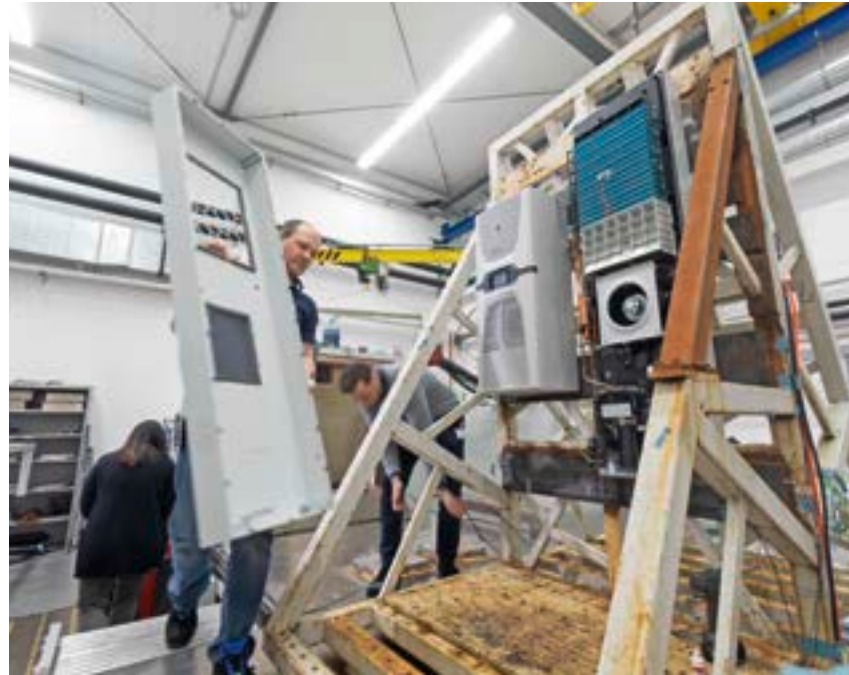
Vibration test: The units are attached to a vibrating plate. The tests are conducted on various axes to simulate impacts from different directions.
