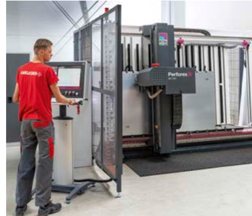
Left: Eplan Smart Wiring visualises every step in the wiring process. Above: The Perforex drilling and milling centre from Rittal automates enclosure machining.
