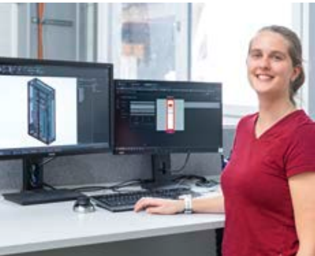
Above: The digital twin of the enclosure is created in Eplan Pro Panel. It includes all the necessary information for downstream processes and makes this available for each subsequent process step.
