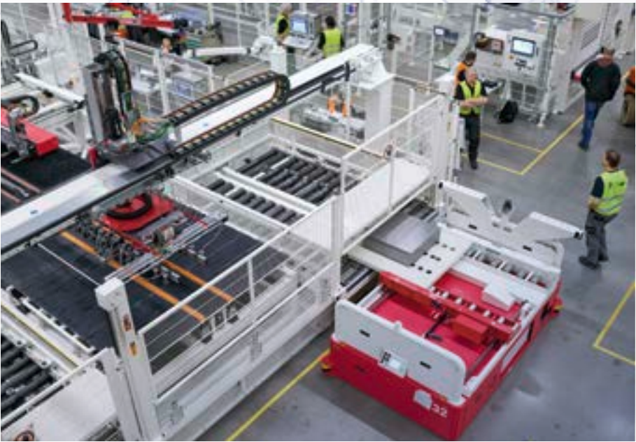
The Rittal plant in Haiger: Every day, around 8,000 compact enclosures are manufactured here using highly automated processes.
